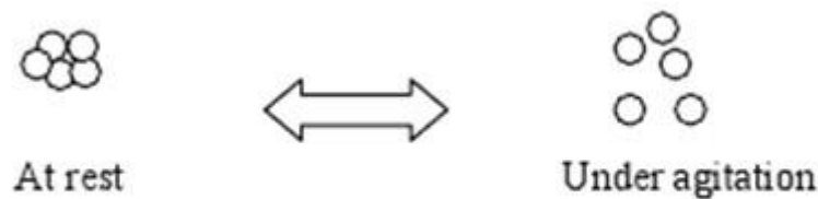
Figure 2- 8.Physical description of the thixotropic behavior of cementitious materials [48]
